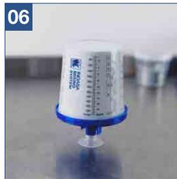
06 Use the cap or flat lid to seal and protect the remaining material in accordance with recommendations of the paint manufacturer and with local regulations or authorities.
