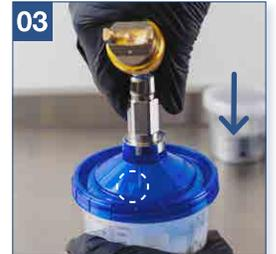
03 Select the right adapter, align the spray gun with the arrow and push down until firmly in place.
