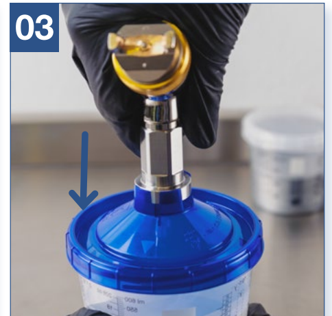
03 Select the right adapter, align the spray gun with the arrow and push down until firmly in place.
