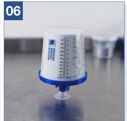
06 Use the cap or flat lid to seal and protect the remaining material in accordance with recommendations of the paint manufacturer and with local regulations or authorities.
