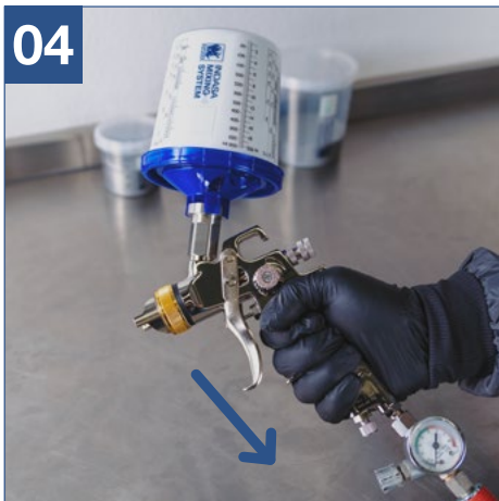
04 Disconnect air line. Invert gun and pull trigger to release excess paint.
