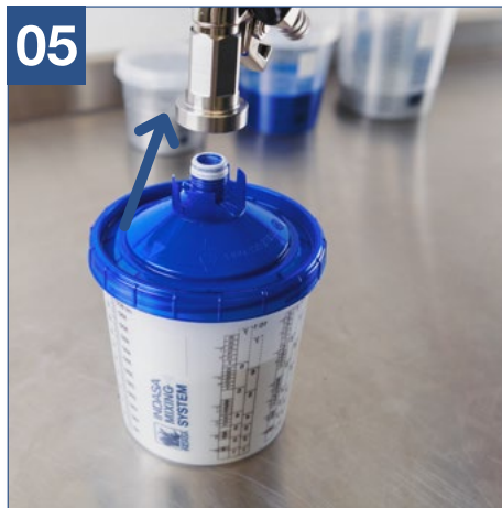
05 Pull the spray gun upwards to disconnect cup from the spray gun.
