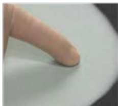
Micro-porosities are nearly invisible and often lead to painting defects
